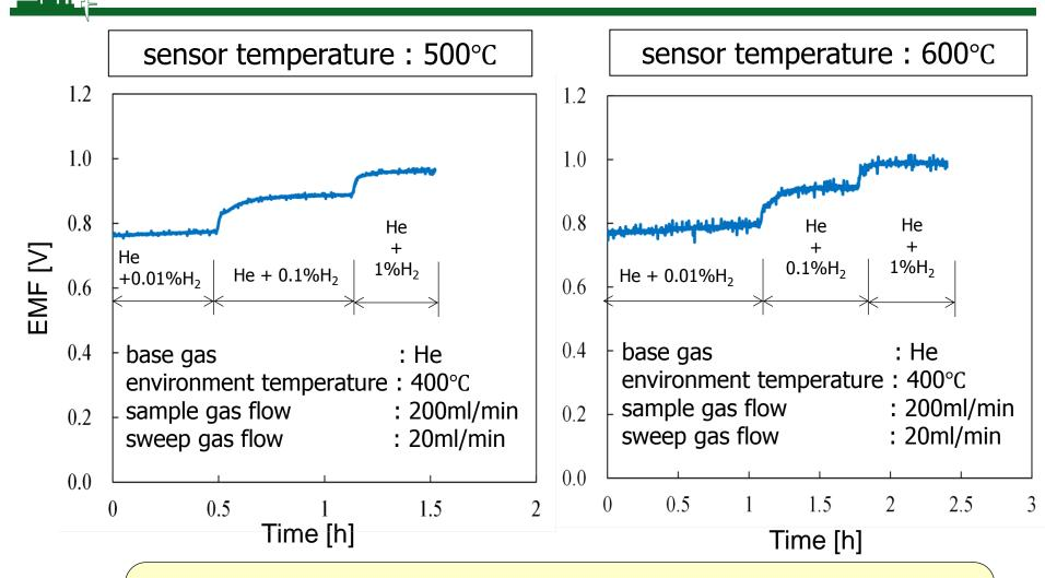
EMF of the hydrogen sensor was increased with  $H_2$  concentration change at each temperature
