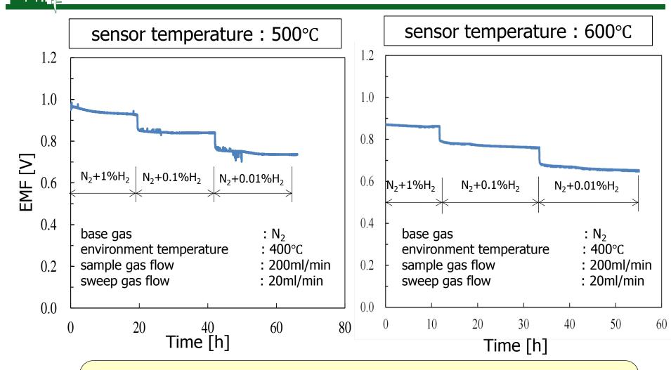
EMF of the hydrogen sensor was decreased with  $H_2$  concentration change at each temperature
