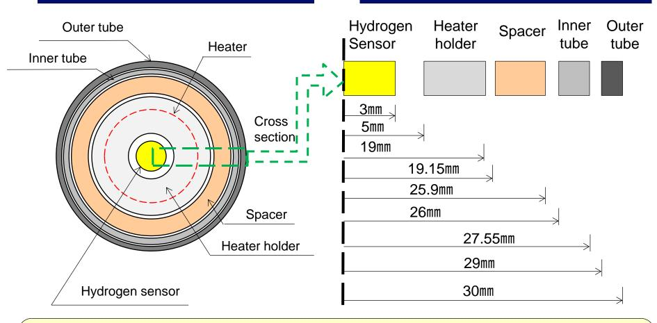
Inner temperature of the irradiation capsule was estimated by GENTC code to confirm the fabricated capsule is possible to heat the hydrogen sensor up to 400~600°C
