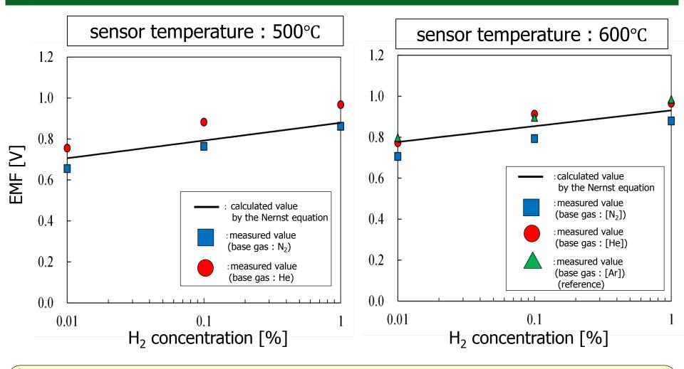
It was found that the hydrogen sensor was able to measure  $H_2$  concentration with high accuracy in each base gas conditions.
